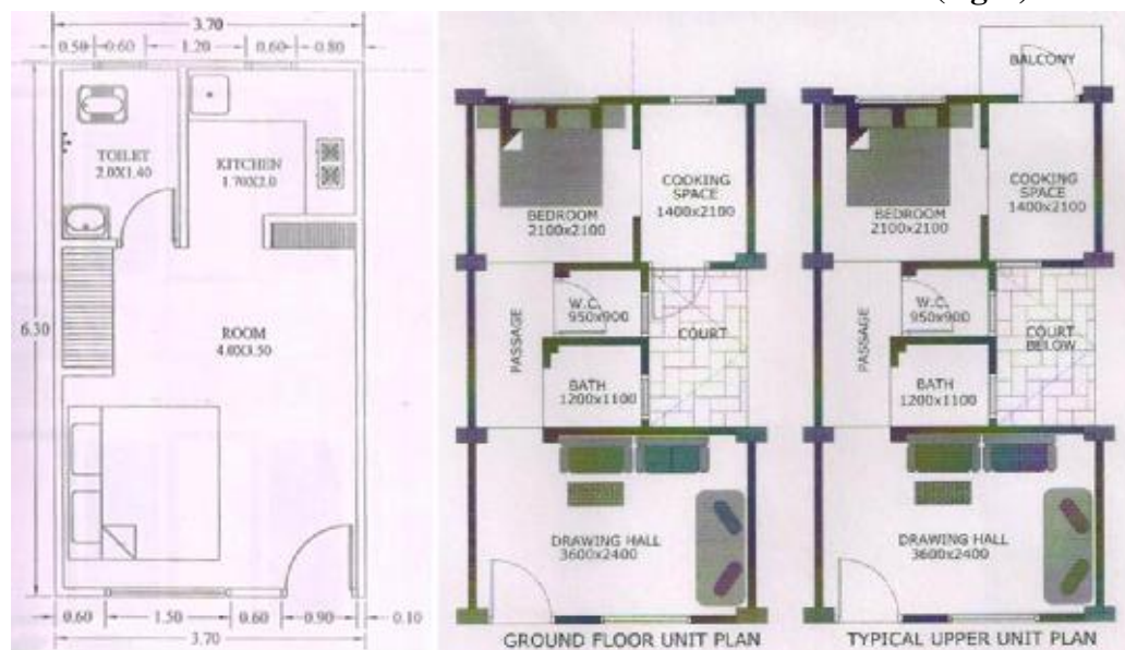
Figure 4: Unit Plan proposed initially (left) and Unit Plan changed to accommodate two rooms and kitchen in the same area (right)
