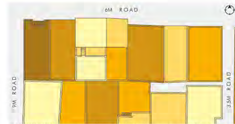
ROOF PLAN, 1:200, It's a juxtaposition of varying building heights from single storyed to four-five floors, mostly built wall-to-wall, there is no room for setbacks.
